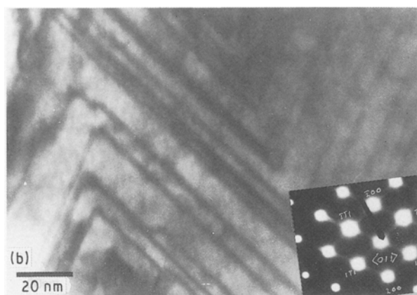
Figure 2 Isolite whiskers. (a) Transmission electron micrograph showing a small-angle grain boundary and the presence of the characteristic chevron defect markings. (b) Higher magnification TEM image of the chevron defects, with inset diffraction pattern showing streaking perpendicular to the defect planes.
