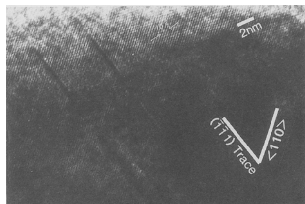
Figure 4 High-resolution transmission electron micrograph of the defects in the chevron region show very narrow stacking faults.
